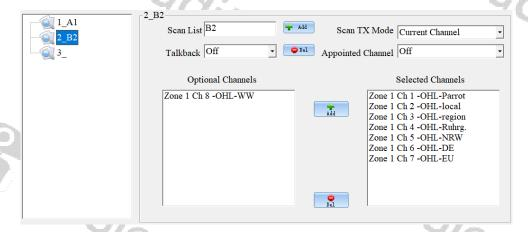
Note: When Scanning is turned on and VFO A is currently selected, the radio will no longer monitor VFO B. When Scanning is turned on and VFO B is currently selected, the radio will no longer monitor VFO A.
