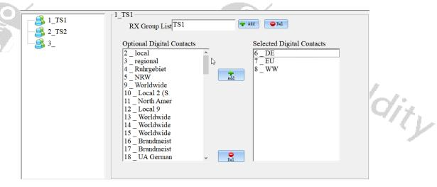
Within the Channel settings a RX Group should be assigned to each channel.
