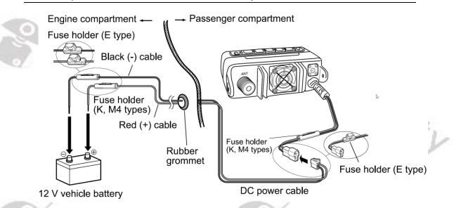
**Notes:** If you use the Radioddity DB25-D for a long period and the vehicle battery is not fully charged or when the car engine is OFF, the car battery may become discharged and will not have sufficient power left to start the vehicle. Avoid using the Radioddity DB25-D in these conditions.
