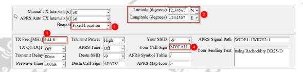
Furthermore, set the analog APRS reporting frequency (3) according to your local requirements. For the US that frequency is 144.3900 MHz, for Europe it is 144.8000 MHz. For all other countries see the details on 'TX Freq [MHz]' regarding that parameter.
