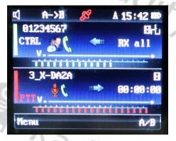
Whenever a digital signal is been received, the DMR ID of the received station will be shown on the left of the receiving VFO
