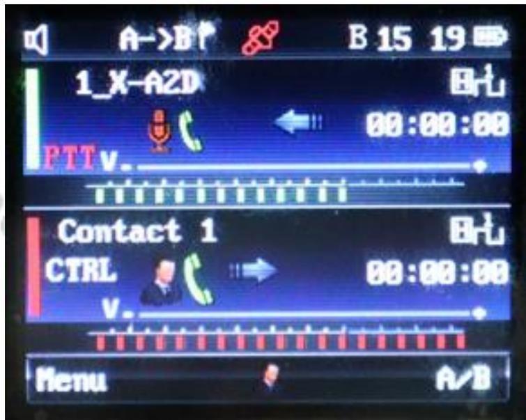
**Notes:** If no contact has been selected for the digital output channel, repeating will fail and a message, stating 'No Contact' will be displayed on the radio screen.
