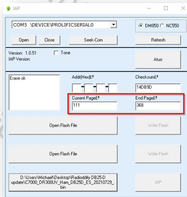
18. As soon as the update has finished on the Radioddity DB25-D, the radio will automatically shut down, whereas the Radioddity GD-88 will state the following on its screen 'Status: Rec Done!'. If you have just updated one of the two GD-88 VFOs it is now time to select the second VFO (long press of the upper side key) and update it with its corresponding firmware file as well. After you have updated both VFOs of the Radioddity GD-88 turn off the radio.
