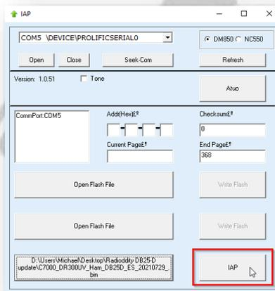
17. Do not press any key on the radio, do not remove power, just wait until the radio has finished the update process and turns off! During the update process, the status-LED will flash green and red and the application shows the progress by the increasing number of 'Current Page'.
