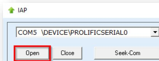
12. If the updater can connect to your Radioddity DB25-D or GD-88, it will output 'IAP Successfully'. If it isn't able to connect to the radio, it will stay on 'CommPort:COMx' (where 'x' represents the selected virtual COM-port number of your programming cable). If you forgot to shut down the CPS, you will get a 'The COMM port is occupied or doesn't exit!' error.
