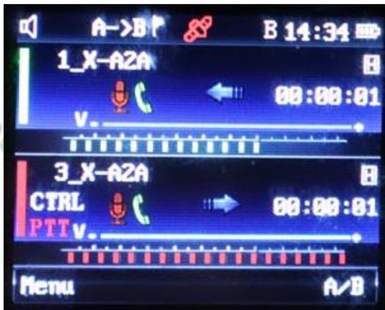
**Notes:** If a channel is set for CH mode of 'Analog', Relay mode will not be available for that channel. That's why it needs to be set to 'A&D, TX-A' for cross-band repeating to work.
