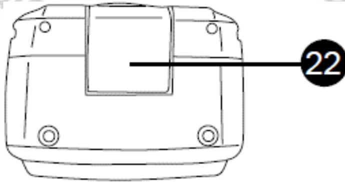
To remove the battery, turn off the radio, clip open the battery latch and then remove the battery by lifting it up, starting with the bottom side. Next carefully move it off the upper metal. Avoid breaking the battery noses.
