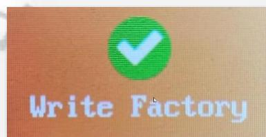
As soon as all data has been transferred from the CPS to the Radioddity DB25-D or GD-88, the text 'Write Factory' will disappear.
