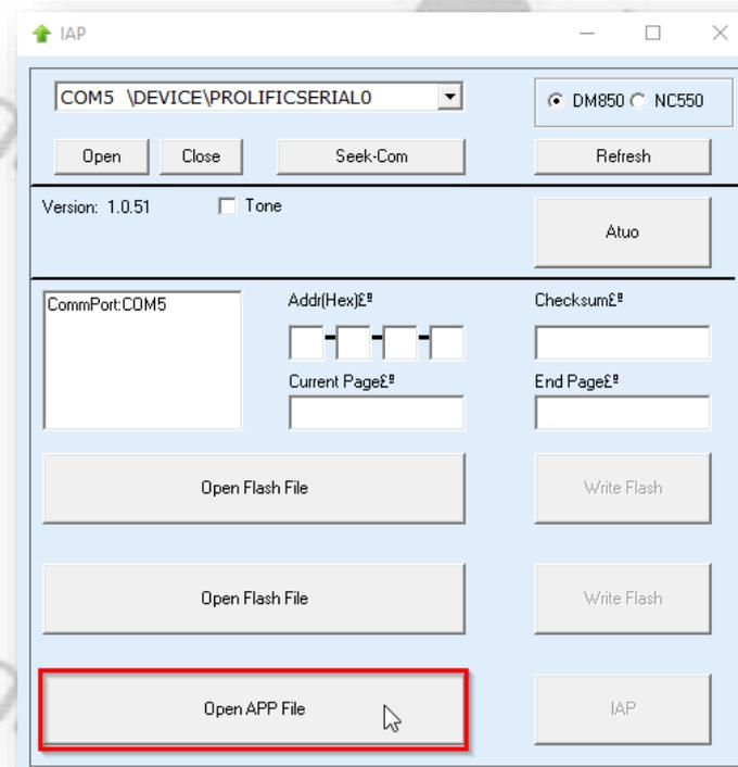
14. Now navigate to the path that does contain the update file that is intended to be transferred to the Radioddity DB25-D or Radioddity GD-88, such as:
