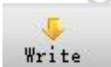
To save the 'Contact list' to the radio, click on 'Write' within the top menu selection of the CPS. Do not forget to do that.
