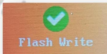
As soon as all data has been transferred from the CPS to the Radioddity DB25-D or GD-88, the text 'Flash Write' will disappear.
