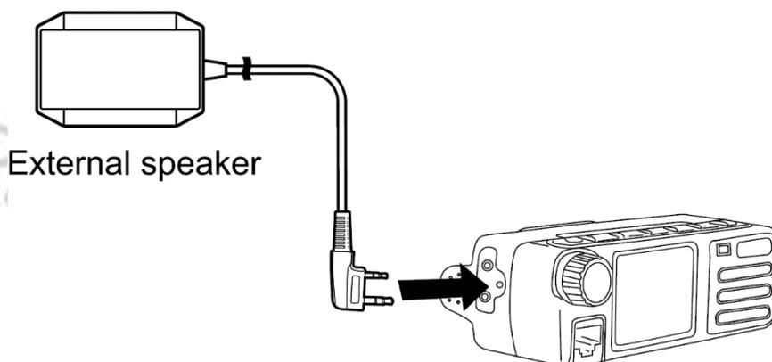
The radio has two jacks (K1 style) for speaker and microphone. Please refer to the instructions to determine how to use an external speaker or headset and microphone accessory. On the Radioddity DB25-D those are on the left side and covered by a small door that's fastened to the radio with a screw. On the Radioddity GD-88 those ports are on the right side and covered by a rubber cover.
