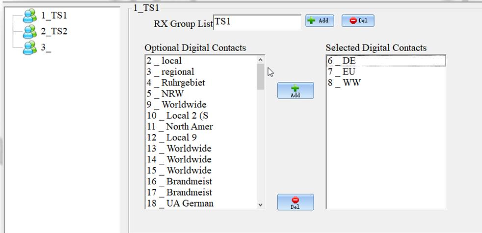
Within the Channel settings a RX Group should be assigned to each channel.
