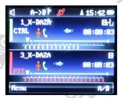
Whenever an analog signal is been received, only the channel name will be shown on the left of the receiving VFO
