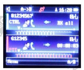
The DMR ID of the received station will be shown on the left of the receiving VFO. Depending on the use of DMR ID Data and/or Talker Alias, additional details may be shown.
