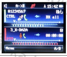
Whenever a digital signal is been received, the DMR ID of the received station will be shown on the left of the receiving VFO. Depending on the use of DMR ID Data and/or Talker Alias, additional details may be shown.
