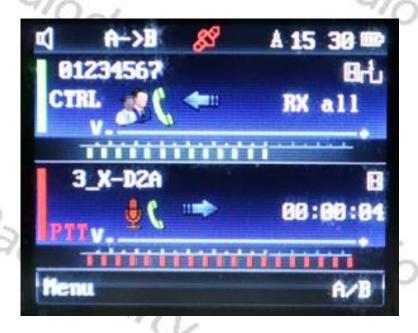
The Radioddity GD-88 will digitally receive on VFO-A (144.100 MHz), TS 1, CC1 and analog transmit the received signal on VFO-B (433.100 MHz), acting as a digital to analog crossband-repeater.
