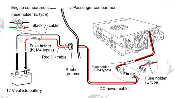
**Notes:** If you use the Radioddity DB40-D for a long period and the vehicle battery is not fully charged or when the car engine is OFF, the car battery may become discharged and will not have sufficient power left to start the vehicle. Avoid using the Radioddity DB40-D in these conditions.
