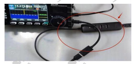
A wired network connection via a LAN adapter connected to the HOST port of Note: the Xiegu X6100 has the advantage that weak Wi-Fi signals and the resulting packet loss are avoided.
