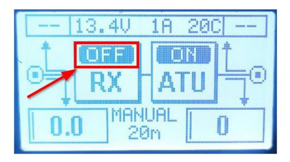
• Switch off the automatic antenna tuner of the Xiegu X6100 (if necessary).
