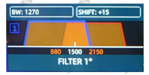
Switching between the low-pass filter shown in blue and the high-pass filter shown in red is done by pressing the MFK rotary knob.
