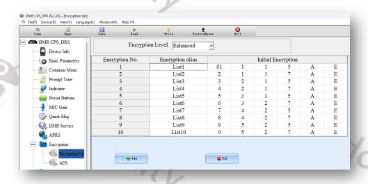
If the Encryption Level is set to AES, the actual encryption key values are defined within the 'AES' submenu underneath the Encryption menu.
