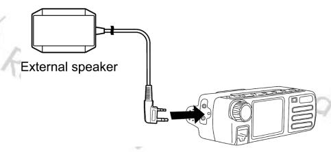
The radio has two jacks (K1 style) for speaker and microphone. Please refer to the instructions to determine how to use an external speaker or headset and microphone accessory. On the Radioddity DB25-D those are on the left side and covered by a small door that's fastened to the radio with a screw. On the Radioddity GD-88 those ports are on the right side and covered by a rubber cover.
