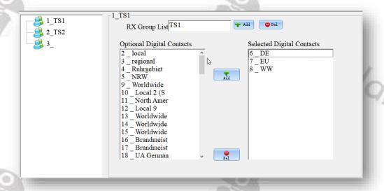
Within the Channel settings a RX Group should be assigned to each channel.
