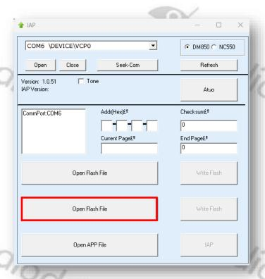
6. Now navigate to the path that does contain the flash file that is intended to be transferred to the Radioddity DB25-D, DB40-D or GD-88, such as:
