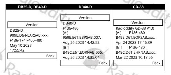
**Notes**: Depending on the Radioddity model and its production run, there may be slight differences in the display of the firmware version even if the very same firmware had been used. However, the stated date and time are unique to each file. Never mix files that are not intended for your radio. As for the Radioddity DB40-D and Radioddity GD-88 only use file-pairs that have been distributed by Radioddity within the very same archive.
