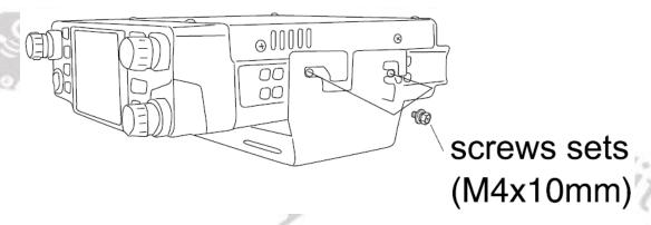
4. With the rotatable fixed point on the left and right sides of the Mounting Bracket, it can tilt the main body at an appropriate angle.
