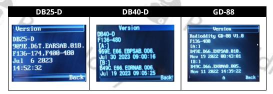
**Notes**: Depending on the Radioddity model and its production run, there may be slight differences in the display of the firmware version even if the very same firmware had been used. However, the stated date and time are unique to each file. Never mix files that are not intended for your radio. As for the Radioddity GD-88 and Radioddity DB40-D only use file-pairs that have been distributed by Radioddity within the very same archive.
