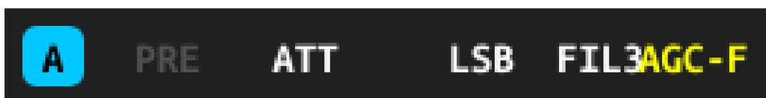
4. Press and hold the [PRE] button again to switch the attenuator off again. The **ATT** label in the 'Status 3' field is then grayed out to indicate that the attenuator is switched off.
