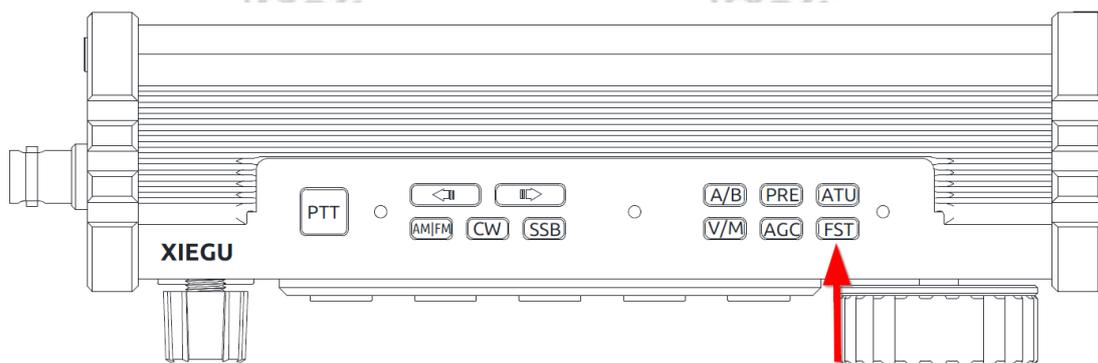
3. Then use the large rotary knob to change the operating frequency which will jump in the set frequency step width.
