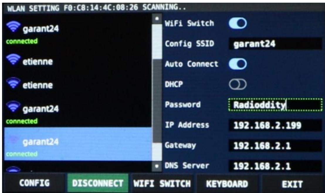
You can confirm connection by the fact that 'connected' now appears in green below the Wi-Fi SSID. In addition, the labeling of the second softkey has changed from 'CONNECT' to 'DISCONNECT'.
