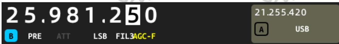
If you press and hold the [A/B] button (this corresponds to the 'A=B' function), the current frequency and mode in the main frequency display (regardless of which VFO it is assigned to) is also transferred to the other VFO.
