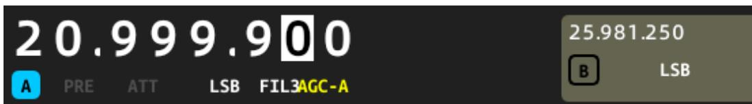
Split frequency operation can also be activated/deactivated via the 'RADIO SETTINGS2' submenu. However, this is much more complicated than a long press on the [AGC] button. Split mode is most often used when calling a DX station in a pile up when you should not transmit on the same frequency as the DX station. Further details can be found in section 10.1.2.3 SPLE on page 43.
