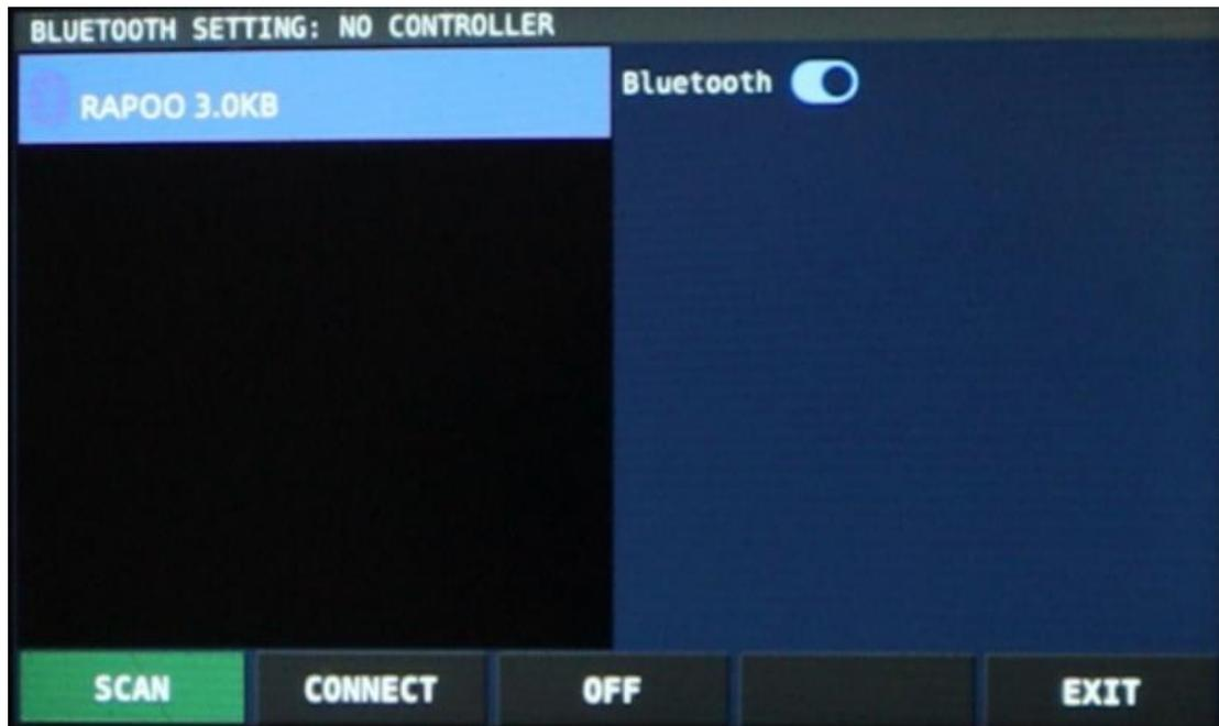
For successful pairing between the Bluetooth device and the Xiegu X6100, the Bluetooth device must be in pairing mode. As soon as the device has been successfully paired with the Xiegu X6100, "paired, connected" will be shown in green underneath the name of the Bluetooth device.
