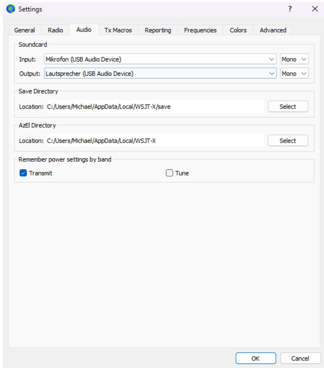
If all is setup correctly you should be able to decode digital signals. In order to make a QSO with another station you have to manually enable TX by clicking the 'Enable TX' button. The function will automatically be deactivated as soon as your QSO has been completed or the TX watchdog has kicked in.
