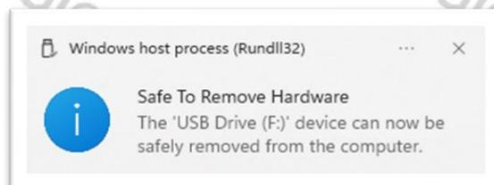
**Note:** Never remove the microSD/flash memory card from the PC without first 'ejecting' it.
