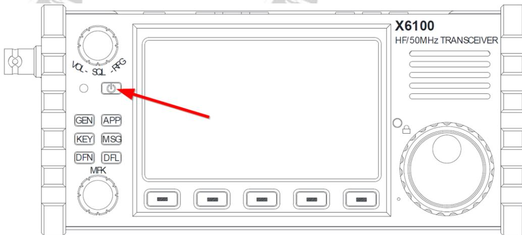
3. The operating system (APP) updates itself automatically after the radio is switched on without the need for manual intervention. After about 2 minutes, the update process is completed and the shutdown message prompt appears on the screen, after which the Xiegu X6100 shuts down automatically.
