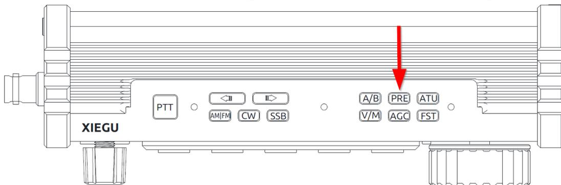
1. Briefly press the [PRE] button on the top of the Xiegu X6100. The **PRE** label will then appear in the 'Status 3' field to indicate that the preamplifier has been switched on.
