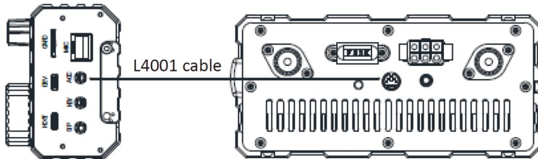
The Xiegu X6100 automatically switches the frequency band of the Xiegu XPA125B, so the operator can concentrate on the controls on the X6100. ALC control is performed between the two devices, so that if the output power of the Xiegu X6100 exceeds the input power limit of the Xiegu XPA125B the ALC control automatically reduces the output power of the Xiegu X6100 hence the output power of the Xiegu XPA125B is maintained safely at around 100 W.
