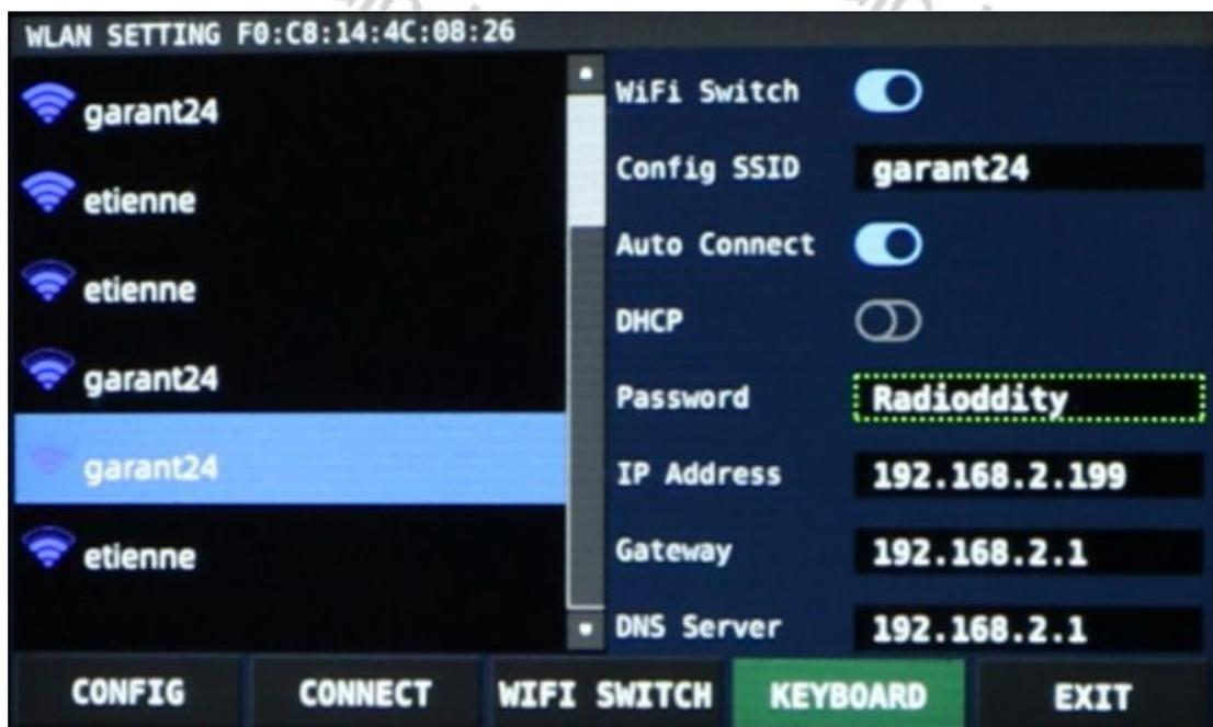
Then press the 'CONNECT' softkey to connect the Xiegu X6100 to your local Wi-Fi. After a few seconds, it will have logged into the local Wi-Fi network.
