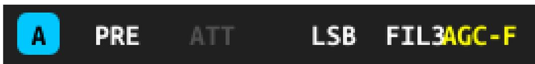
2. Briefly press the [PRE] button again to switch the preamp off again. The **PRE** label in the 'Status 3' field is then grayed out to indicate that the preamplifier is switched off.
