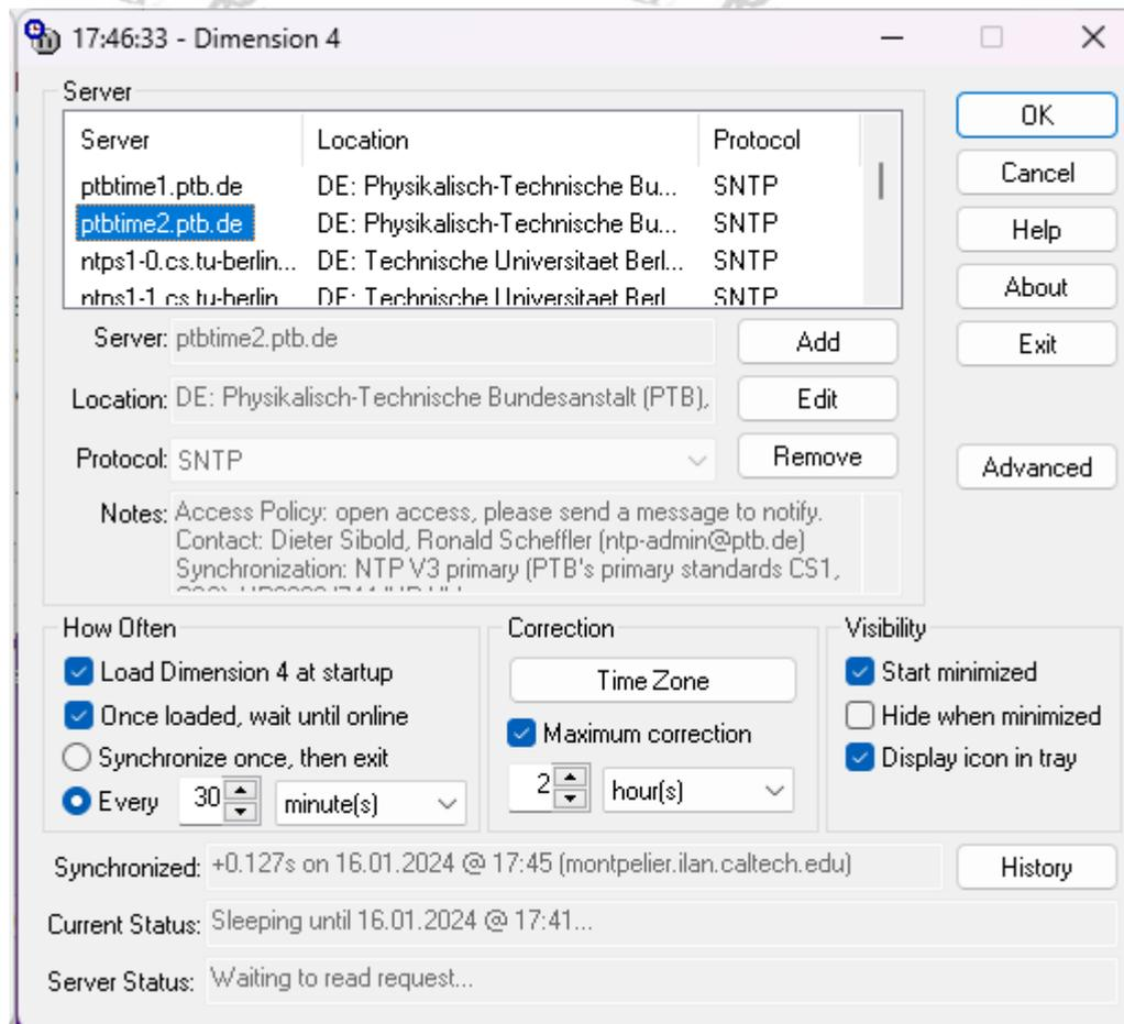
In the above example it is setup to synchronize the internal PC clock against ptbtime2.ptb.de every 30mins.
