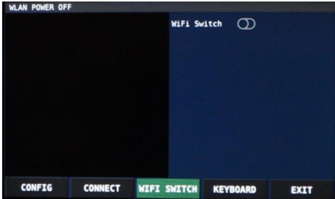
As soon as Wi-Fi has been activated, the Xiegu X6100 automatically searches for available 2.4 GHz Wi-Fi networks. It then lists all found networks on the left-hand side. By turning the MFK knob you can scroll through the list of SSIDs found. If you have a mesh network, the same SSID may be listed several times.
