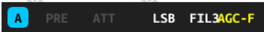
3. However, if you press and hold the [PRE] button on the Xiegu X6100, the label **ATT** will appear in the 'Status 3' field to indicate that the attenuator has been switched on.
