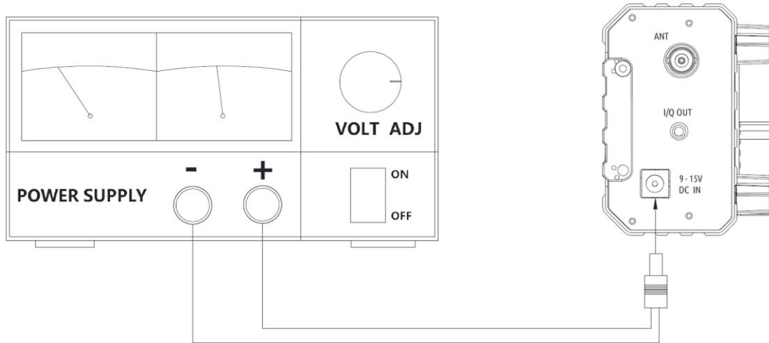
To prevent external interference from entering the radio via the power lines and to prevent radio frequency interference in the radio from being radiated to the outside via the power lines when the Xiegu X6100 is operated with an external power supply, additional Clip-on EMC ferrite rings can be attached to the DC supply cable. If possible, the ferrite rings should be attached close to the radio.
