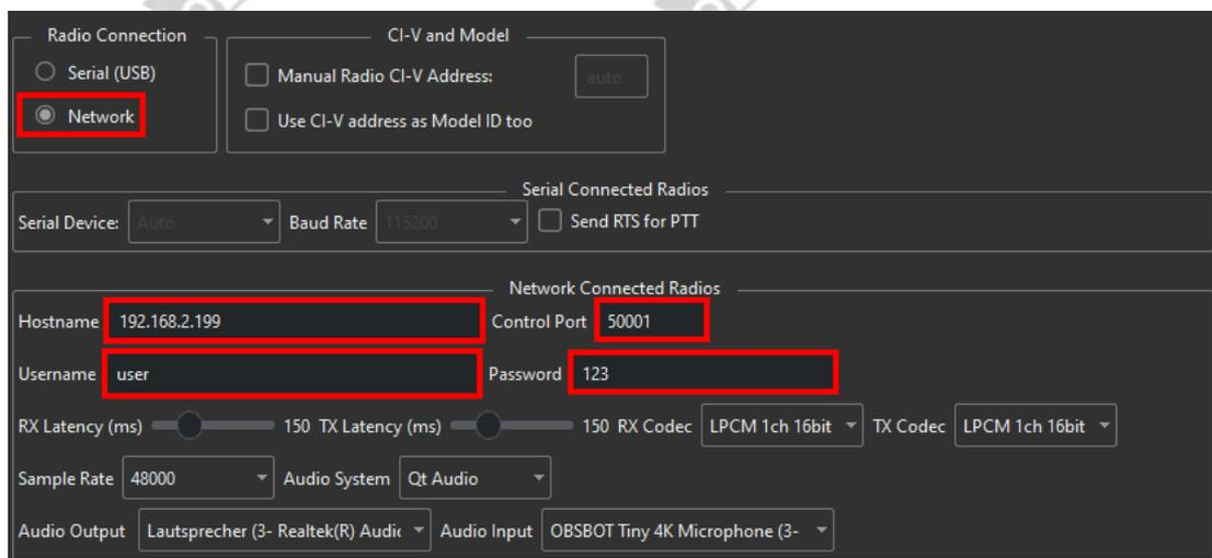
You should then check the audio output and input settings for wfview running on your computer. These can be found under the heading 'Audio Output' and 'Audio Input' below the previously adjusted communication settings.
