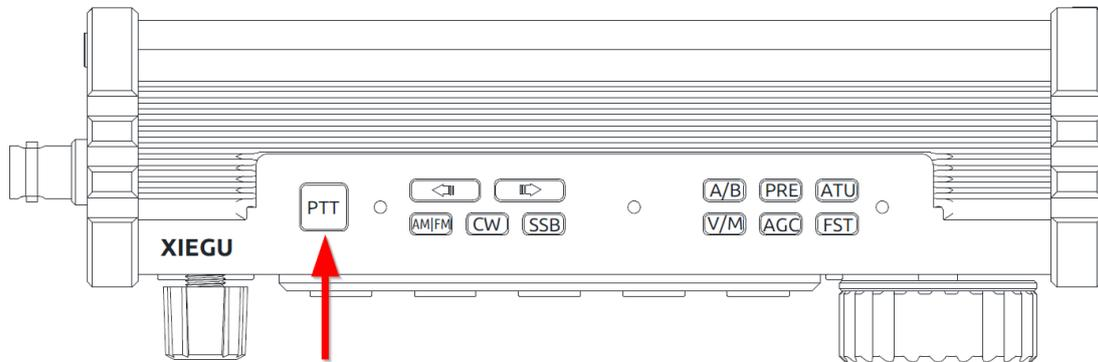
1. Press the [PTT] button on the top of the device and speak into the built-in microphone opening to the left of the large knob to transmit your voice.
