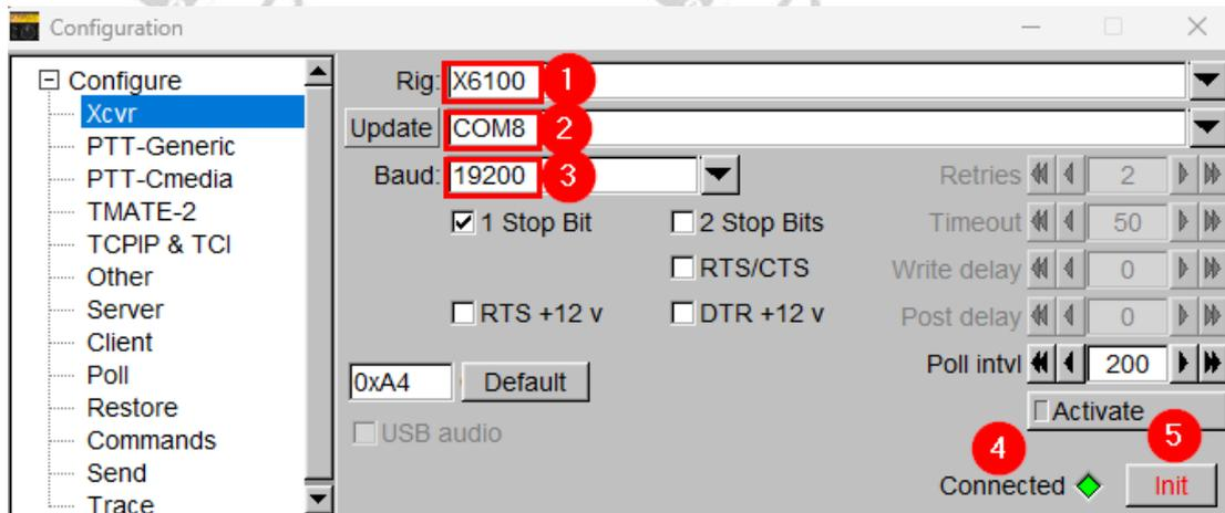
You will hear some noise of the solenoids inside the Xiegu X6100. After the initialization sequence has finished, the 'Init' label of the button (5) should no longer be printed in red, but black and the LED-indicator (4) should be colored green.
