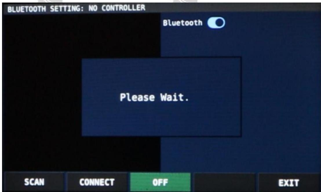
Now use the MFK rotary knob to select a device from the devices listed on the left-hand side and confirm your selection by pressing the 'CONNECT' softkey.
