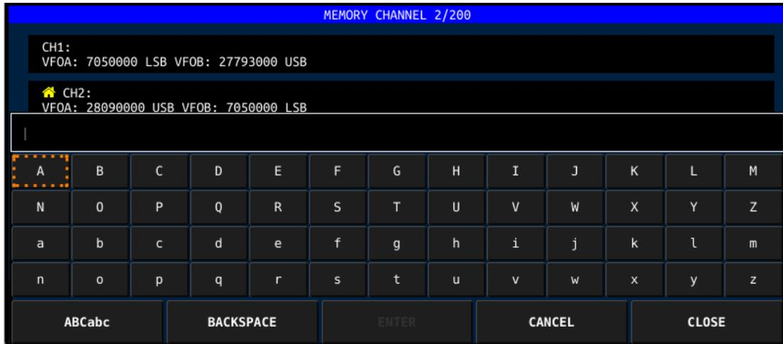
Now enter a name for this storage location. Labelling channels makes it much easier for you to select the correct storage location by name at a later date.
