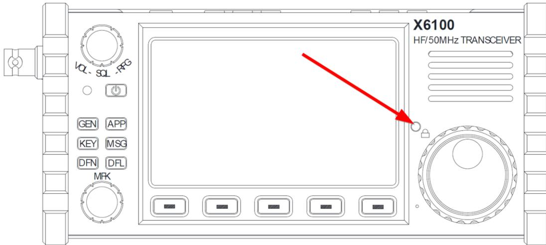
1. Press and hold the lock button to disable the change of using the large rotary knob. The symbol
