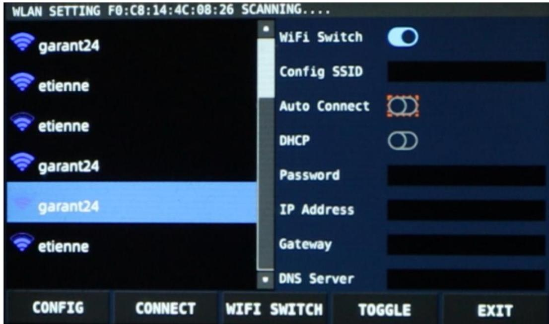
Before you can use any of the networks found, you need to specify the required configuration settings for the specific network. When ever you hit the 'CONFIG' softkey, the settings of the currently highlighted network will be displayed on the right-hand side.
