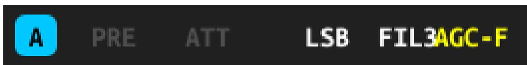
It is recommended not to use the preamplifier in the frequency bands below 14 MHz so that the radio is set to the straight-through state, which improves front-end performance of the receiver and reduces the effect of interfering signals.
