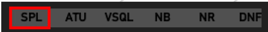
When split frequency mode is switched off (**SPL** is shown in gray in the 'Status 1' field), the two VFOs can be used completely independently of each other and you can switch between the two VFOs by briefly pressing the A/B button on the top of the Xiegu X6100. The operational VFO is displayed as the main VFO frequency.
