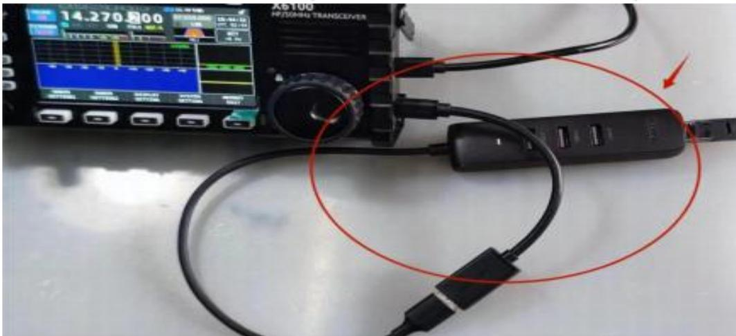
**Note:** A wired network connection via a LAN adapter connected to the HOST port of the Xiegu X6100 has the advantage that weak Wi-Fi signals and the resulting packet loss are avoided.
