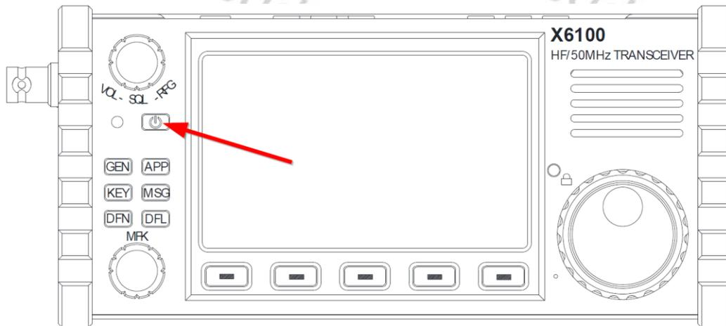
9. To check whether the baseband firmware update was successful, press the following buttons in succession [GEN] → SYSTEM SETTING to access the system settings menu.
