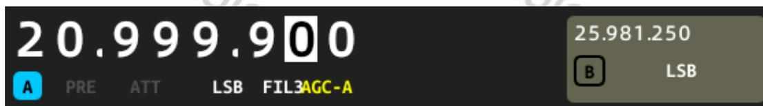
It is much easier to activate/deactivate split frequency operation by pressing and holding the [AGC] button. Details on this can be found in section 9.10 Automatic gain control / split-frequency operation (AGC / SPL) on page 33.
