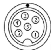
Pins as seen when looking onto the 6-pin socket of the Radiodity QT80
