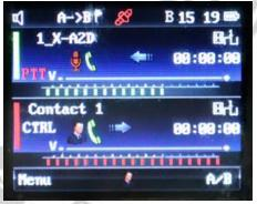
**Notes:** If no contact has been selected for the digital output channel, repeating will fail and a message, stating 'No Contact' will be displayed on the radio screen.
