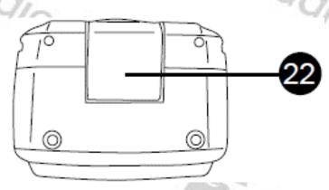
To remove the battery, turn off the radio, clip open the battery latch and then remove the battery by lifting it up, starting with the bottom side. Next carefully move it off the upper metal. Avoid breaking the battery noses.
