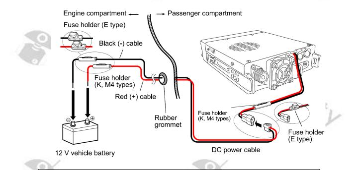
**Notes:** If you use the Radioddity DB40-D for a long period and the vehicle battery is not fully charged or when the car engine is OFF, the car battery may become discharged and will not have sufficient power left to start the vehicle. Avoid using the Radioddity DB40-D in these conditions.
