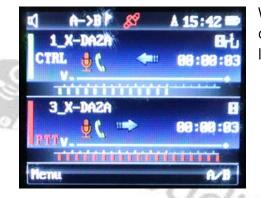
Whenever an analog signal is been received, only the channel name will be shown on the left of the receiving VFO.
