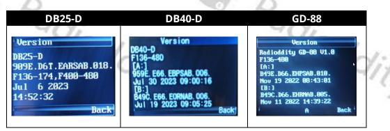
**Notes**: Depending on the Radioddity model and its production run, there may be slight differences in the display of the firmware version even if the very same firmware had been used. However, the stated date and time are unique to each file. Never mix files that are not intended for your radio. As for the Radioddity GD-88 and Radioddity DB40-D only use file-pairs that have been distributed by Radioddity within the very same archive.
