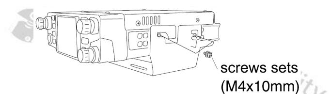
4. With the rotatable fixed point on the left and right sides of the Mounting Bracket, it can tilt the main body at an appropriate angle.
