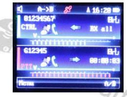
The DMR ID of the received station will be shown on the left of the receiving VFO. Depending on the use of DMR ID Data and/or Talker Alias, additional details may be shown.
