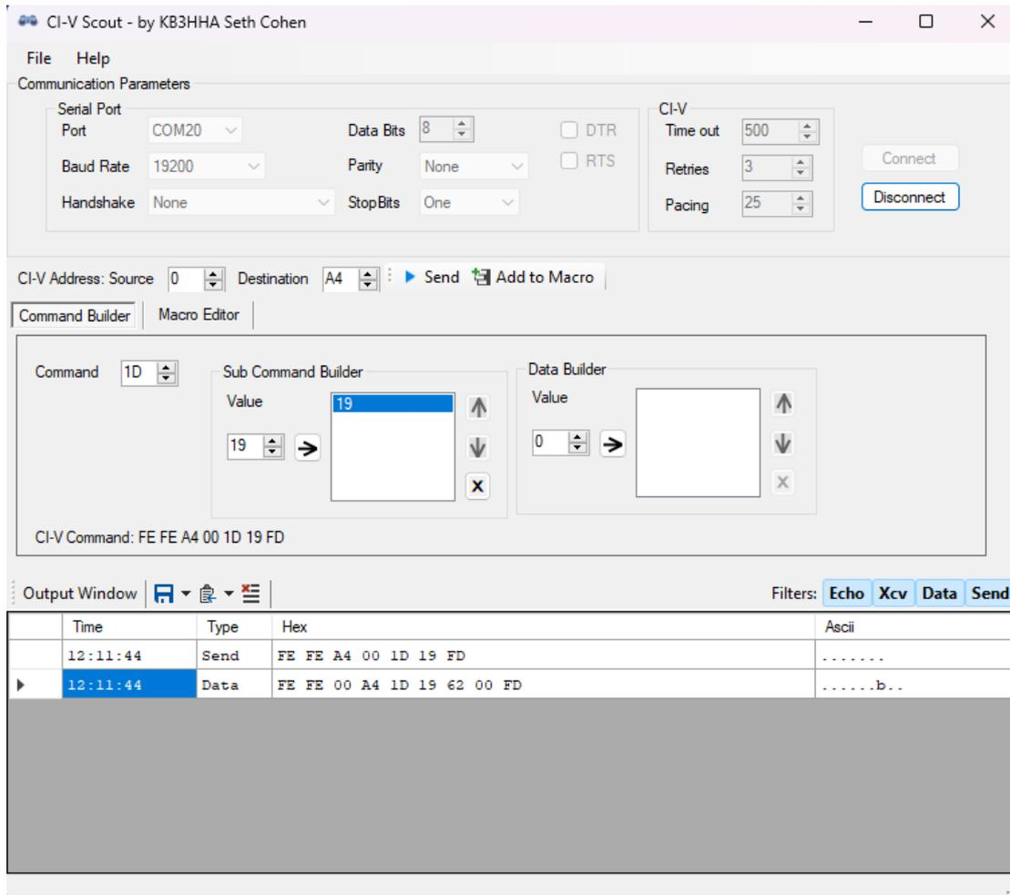
Connect the supplied USB-cable between the Xiegu X6200 DEV port and your PC and setup CI-V Scout to use the com: port corresponding to SERIAL-B of the Xiegu X6200 at a baud rate of 19200bps (to check which port this is use Windows device manager). You can send single commands including subcommands and data to the Xiegu X6200 as well as scripted macros that you create in advance, either manually or through saving individual commands in the program.
