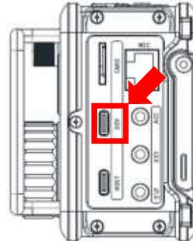
From the PC's point of view, the Xiegu X6200 provides two serial interfaces of the interface chip type CH342. If the CH342 driver is not installed automatically by the host OS, it needs to be installed manually, or the host OS driver tool may be used to install it from the Internet.
