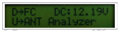
In this mode, it will test and show your antenna system's several parameters, such as SWR, Z, Rs, Jx values. All of these parameters are showed on the LCD.
