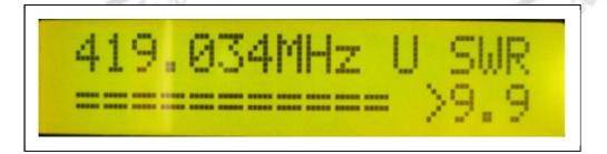
The left example shows the SWR status when no antenna connected to AW07A
