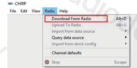
2. Select the corresponding cable driver port, and select Model "BAOFENG Radio" under, then click "OK" to read the radio.
