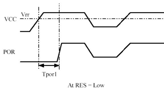
Figure 8-1 Power-On Reset Diagram
