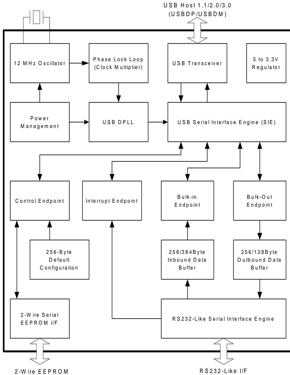
Figure 2-1 Block Diagram of PL2303TA
