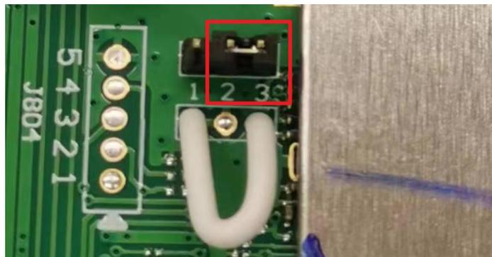
**Step 5.** Cut the J803 wire with a pair of scissors.
