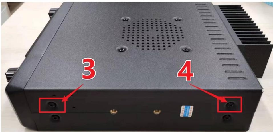
**Step 2.** Remove the top case and be aware of the wired connections on the motherboard.
