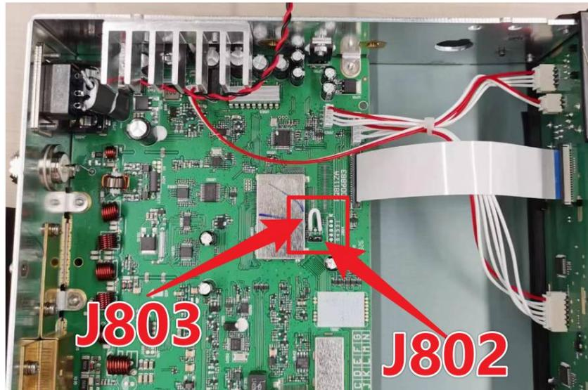
The J802 is covered by a 2-pin connector, bridging 1 and 2 as below.
