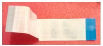
Put some of the Isopropyl-alcohol onto the fabric and wipe from the cable down the silver connections. Turn the cable in order to clean both ends. Only the side with the silver contacts needs cleaning.
