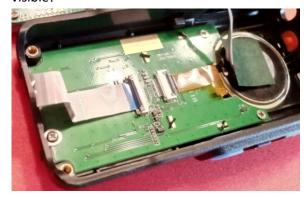
The above picture does show the connector with its latch in the open (upright) position.
