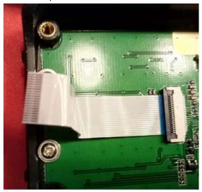
11. Next open the latch of the display PCB (if the connector is to the right and the cable is (normally) routed to the left, then you may use your fingernail to carefully put it on the ribbon cable, facing the fingernail towards the connector. Now carefully lift up the black part of the connector (90°, no more!) in order to open the connector and release the ribbon cable. The silver connectors (on the left) and the blue isolation tape on the rioght should be visible!
