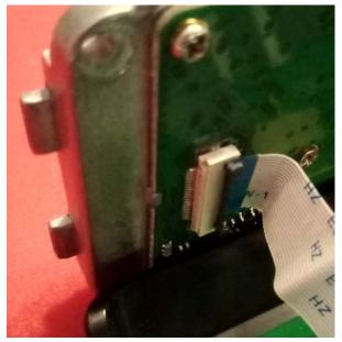
The above picture does show the connector with its latch in the open (upright) position.
