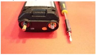
5. Now use the flat screwdriver and carefully remove the two nuts that fix the ON/OFF/Volume and the Antenna to the main body (also by turning them counterclockwise)
