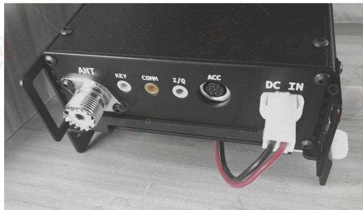
3. Plug the power cord of G90 into the associated interface on the cooling bracket.
