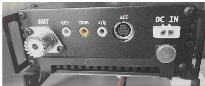
2. Plug the power plug on the cooling bracket into the DC IN socket of G90.
