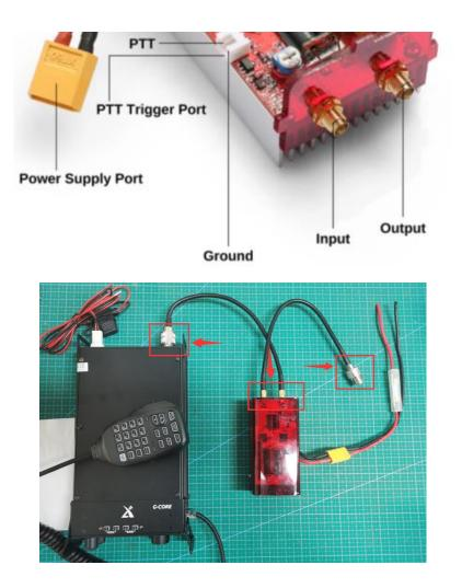
4. Connect the PTT trigger cable C
