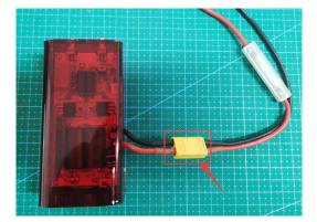
2. Connect to the DC power supply: 13.8V/20A
