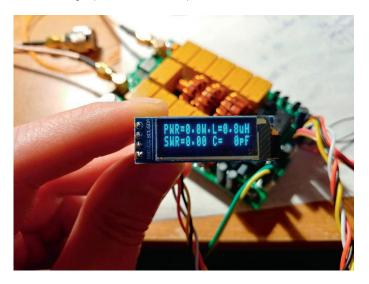
The indication on the 0.91 128x32 display looks like on a regular 1602 display, while having tiny dimensions.
