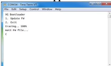
(When updating the main unit, there is a count-down timeout during which time you need to press 1 – when updating the display unit, there is no timeout, it waits for you).
