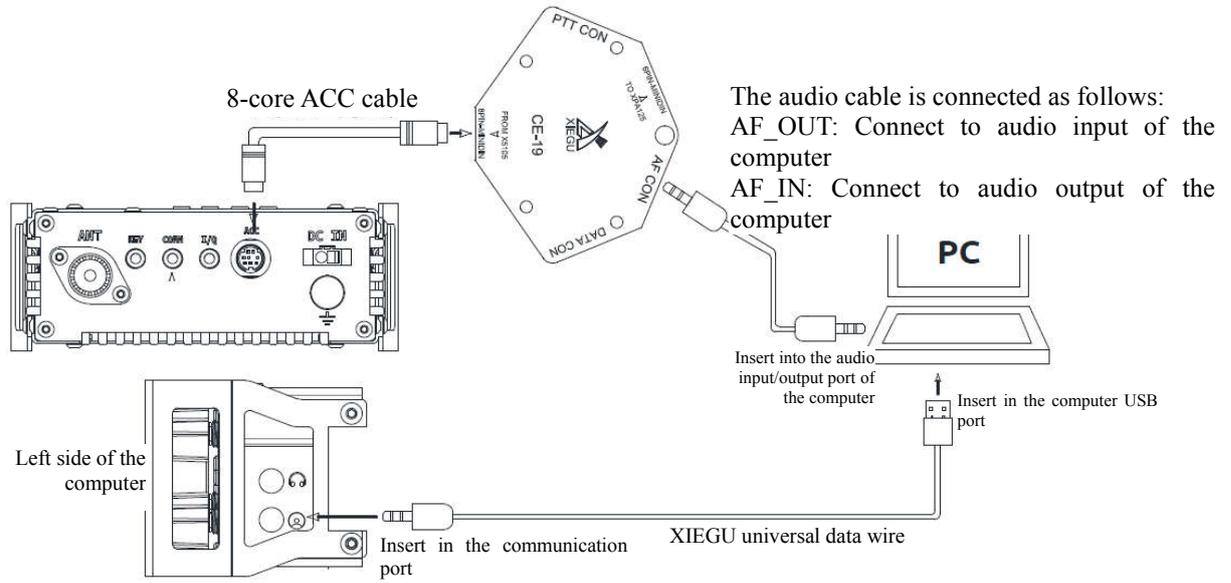
Fig. 1 G90 and Computer Connection Data Communication Diagram
