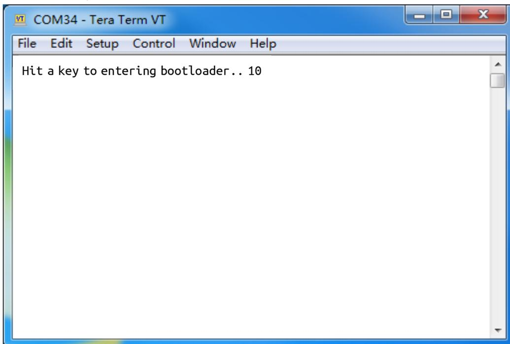
Press SPACE bar on the computer to interrupt the booting procedure.
