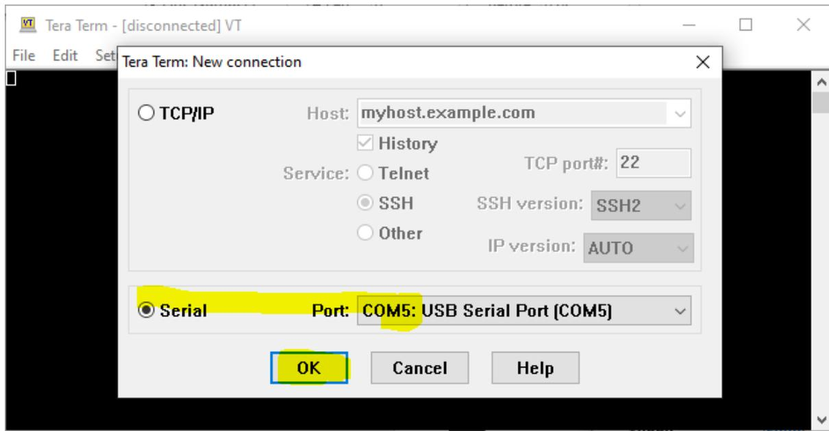
b) Now we set the communications baud rate: Select Setup/Serial port.
