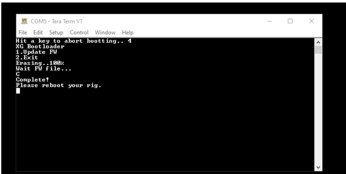
Once the transfer has successfully completed the G90 will restart automatically.
