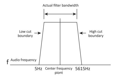
As shown in the figure on the right, the filter consists of L-CUT and H-CUT, and both work together to form an effective filter bandwidth.
