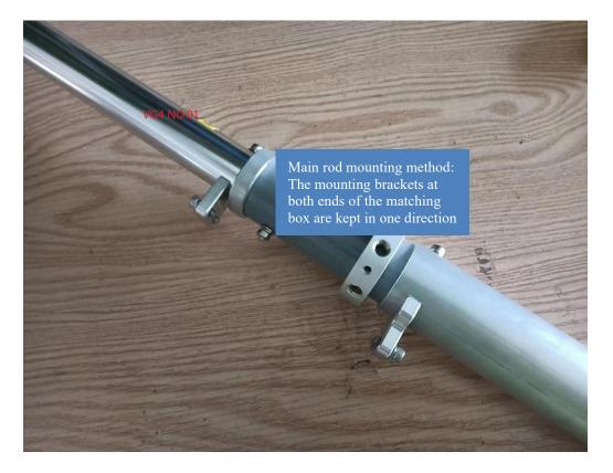
3 Place the matching box on the base support tube and fix it with the supplied screws.
