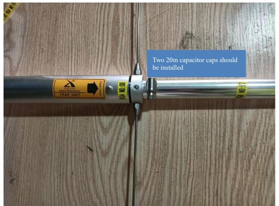
7 Screw in the four 40m capacity hat rods on section NO:9.
