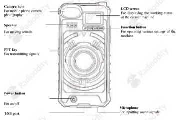
For charging the battery / serving as power bank to charge the phone / reading and writing talkback frequency information
